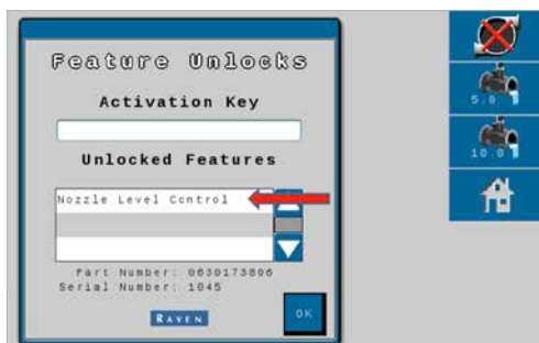
Step 17. If upgrade is successful Nozzle Level Control will be displayed in the Unlocked Features section
