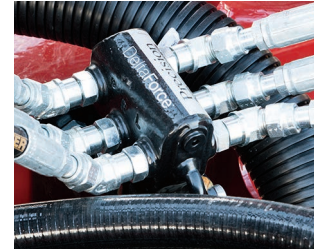
DeltaForce row unit down pressure control
